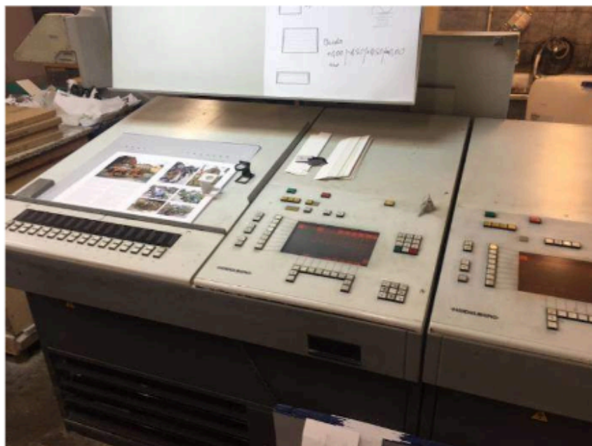
Figure 3: Sistema CPC - Painel de controle com interface digital
